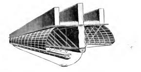
By heating an expansion-chamber the entire machine is made to displace more air than its entire weight, and thus has a lifting power. The centre of gravity is adjusted by means of a moveable weight, and the angle of the aëroplane can thus be adjusted and cause the ascending or descending force to propel the machine ahead. A.D. 1879.
